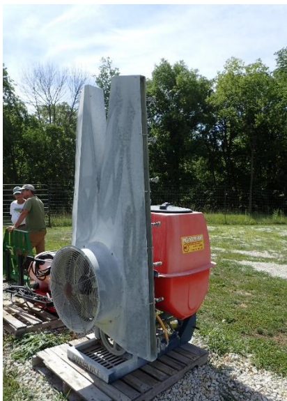
Munckhof 100 gallon 3-point airblast sprayer used to spray dwarf apple trees
