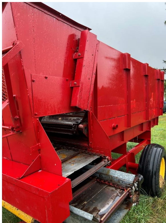
A side view of Deirdre’s locally-made mulch spreader, showing the conveyer which discharges mulch into tree rows.
